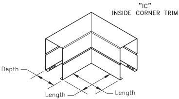
90° ANGLE STANDARD STANDARD LENGTHS 6" X 6" & 12" X 12" REQUIRED 2" MIN. OVERLAP 1 TUBE TO 4 TUBES HIGH
