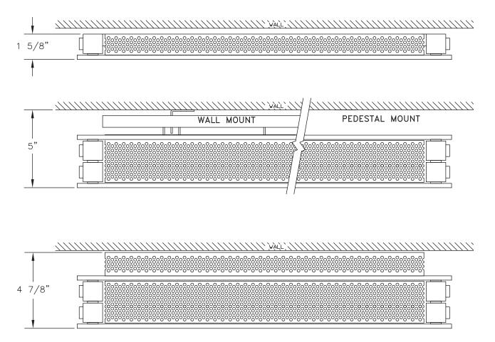
THE 16GA GRILLE WITH 3/16" DIAMETER HOLES ON 1/4" STAGGERED CENTERLINES PROVIDES A PENCIL PROOF FLAT TOP TO ANY STANDARD PANEL. THIS ALLOWS FOR A MORE CONTINUOUS LOOK AND PREVENTS UNWANTED BUILD UP BETWEEN THE FINS. THE GRILLE IS PAINTED AND FINISHED WITH POLYESTER FROXY POWDER TO MATCH THE RADIATOR.
