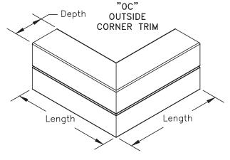
90° ANGLE STANDARD STANDARD LENGTHS 6" X 6" & 12" X 12" REQUIRED 2" MIN. OVERLAP 1 TUBE TO 4 TUBES HIGH
